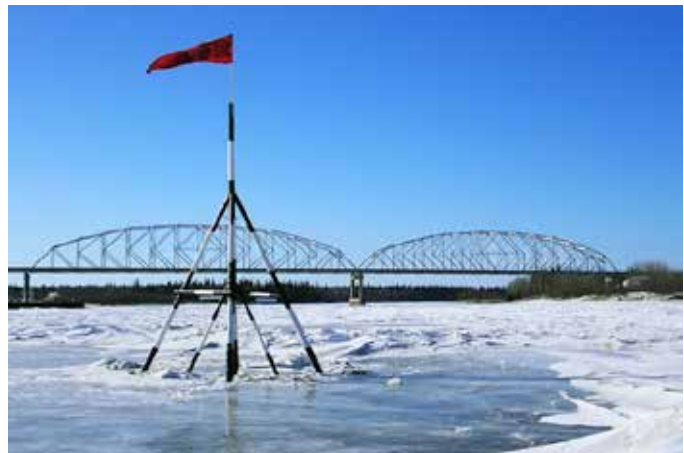
This is the official tripod for the Nenana Ice Classic. The tripod is attached to a clock on the shore by a cable. When the ice under the tripod breaks or starts to move, the tripod moves, pulling the cable and stopping the clock. Photo: James Brooks, https://www.flickr.com/photos/jkbrooks85/3384528606 .
