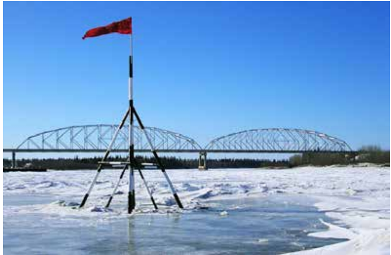
This is the official tripod for the Nenana Ice Classic. The tripod is attached to a clock on the shore by a cable. When the ice under the tripod breaks or starts to move, the tripod moves, pulling the cable and stopping the clock. Photo: James Brooks, https://www.flickr.com/photos/jkbrooks85/3384528606 .
