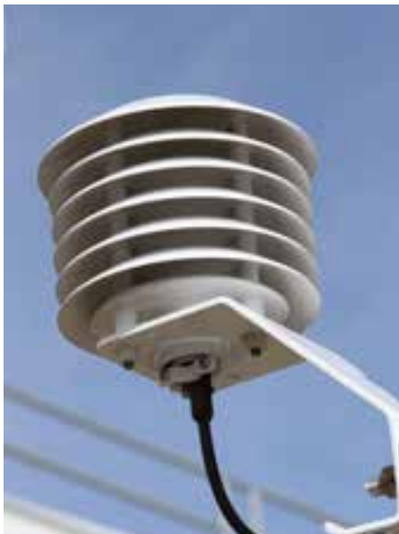
The shield around this temperature sensor protects it from the sun, keeps it dry and provides ventilation. Photo: Yuri Bult-Ito, REACH Up.
