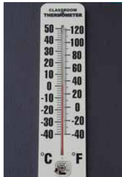
The level of the liquid inside the tube of a thermometer can gauge temperature. Photo: Yuri Bult-Ito, REACH Up.
