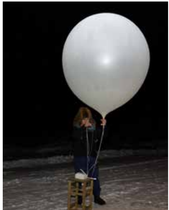
A technician prepares to release a weather balloon that will carry a radiosonde instrument high into Earth's atmosphere. Photo: Geophysical Institute, UAF.
